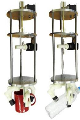
The stiffness of the gripper is adaptable due to weight and rigidity of the object
