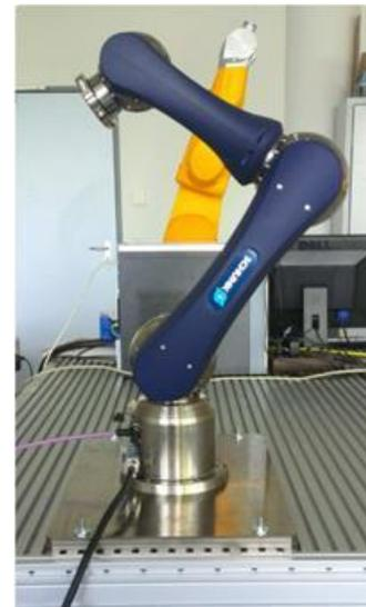
For this class of robots, the change of the system dynamics after reassembling as well as the inherent (passive) compliance of the actuators, result in a source of degradation of the motion control performance. In order to address these challenges, nonlinear model-based control methods are developed paying
