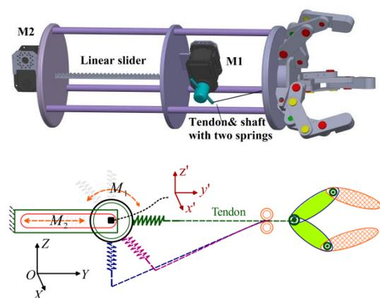
CAD model and schematic design of VSG
