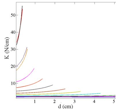
Stiffness of the gripper  $\sigma_0$  in different  $\alpha$ .
